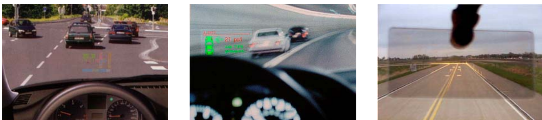
From left to right: HUD from Siemens-VDO incorporated in a BMW, laser scanning HUD from Microvision and a holographic image combiner from Delco Data Vision
